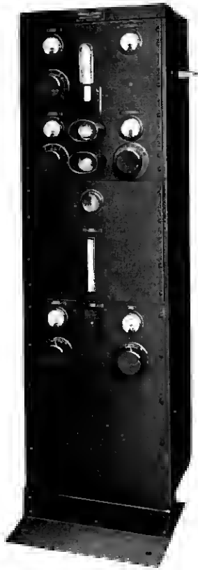
Fig. 3—Front view of crystal controlled oscillator-amplifier unit.
